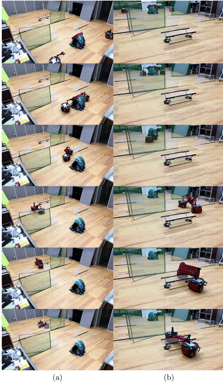
Figure 6.12: Snapshots during the second experiment, taken from two perspectives (a) and (b). The robots start moving towards the pile of clothes (0 sec). Both robots reach the pile simultaneously and grabbing the each tip of the fabric (red checkered blanket) at the top of the pile (20 sec), respectively. In the second experiment, there are two obstacles. The robots avoid the first obstacle (70 sec) and the second obstacle (90 sec) while cooperatively holding the fabric. When they reach the hanger, they stretch the fabric (110 sec) and hang it on the hanger (131 sec).
