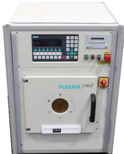
Fig. 2.11 The image of microwave plasma asher which is used for plasma oxidation
