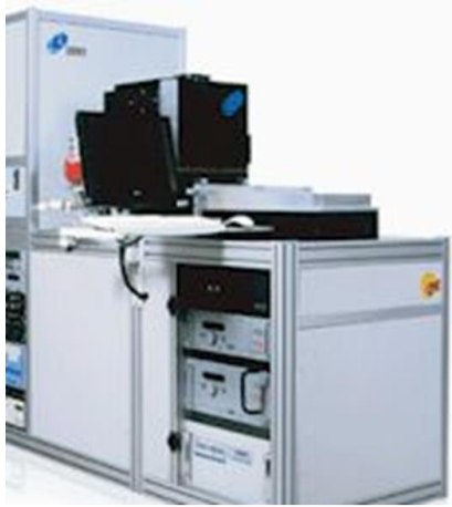
Fig. 2.6 Configuration of the ICP-RIE system in ISRC
