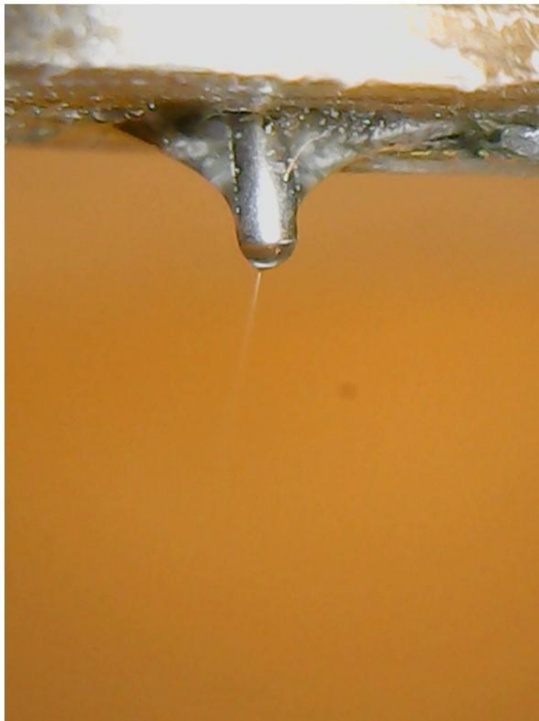
Figure 3-6 Microscopic images of ejected jet. (a) PVP,PEO in ACN and (b) PVP,PEO-AgNO 3 in ACN.
