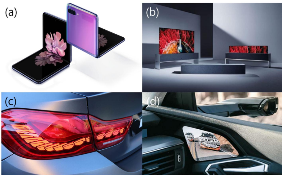
Figure 1.3 Commercial products of OLEDs; (a) Foldable OLED Panel in Samsung Galaxy Z Flip (Samsung Electronics 2020), (b) LG Rollable OLED TV R9 (LG Electronics 2020), (c) OLED lighting in automobile (BMW AG 2017), (d) Virtual exterior mirror (Audi 2018).
