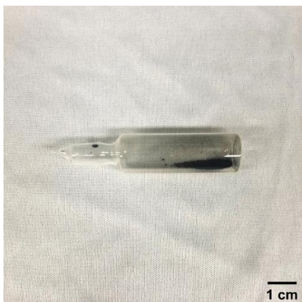
Figure 3.2 Image of sealed glass ampoule. Co-PBAs and sulfur powder were inserted, and the pressure inside was maintained 0.1 Torr.
