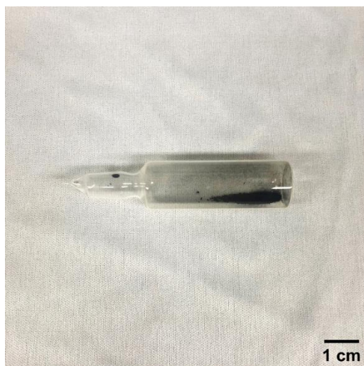
Figure 6.3 Image of sealed glass ampoule. Co-PBA and sulfur powder were inserted. The pressure of ampoule was maintained 0.1 Torr.
