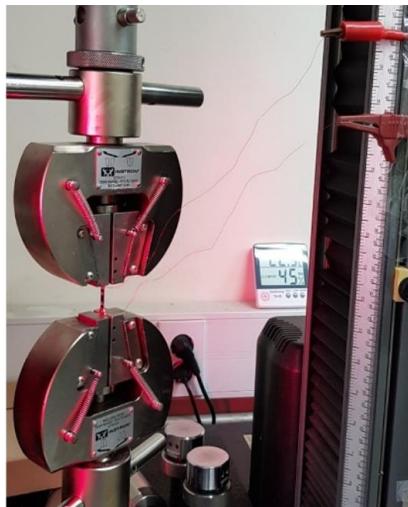
Figure 4-2 Picture of tensile test and stress relaxation test setting. Resistance was measured with Keithley Resistance Meter through copper wire during the test.
