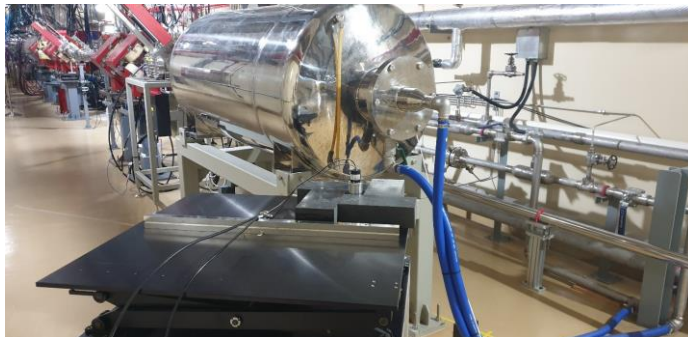
Figure 2.12 Gamma flash detector placed near to the beam dump.
