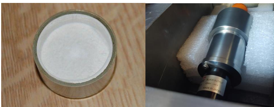
Figure 2.4. (a) 1” LaBr 3 :Ce scintillator crystal and (b) LaBr 3 :Ce gamma detector with R1924A Hamamatsu PMT.
