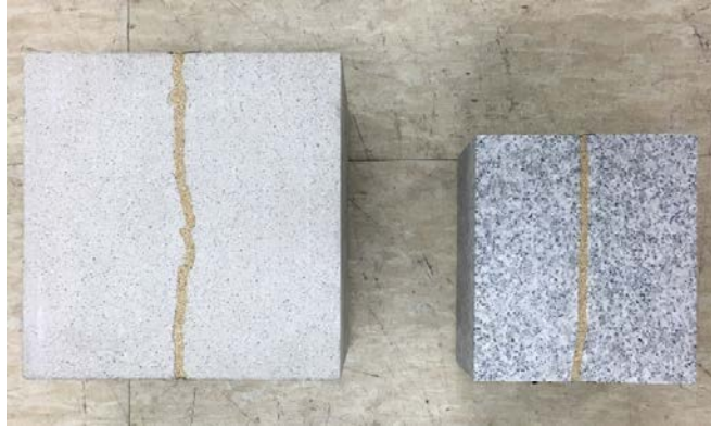
Figure 3.7 Cement mortar specimen (in the left) and granite specimen (in the right) filled with sand at 5mm thickness
