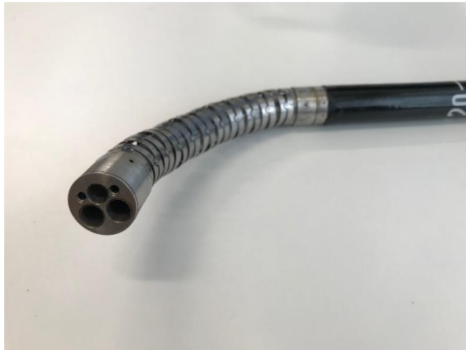
Fig. 2.2 Steerable five-channel overtube with outer diameter 19mm
