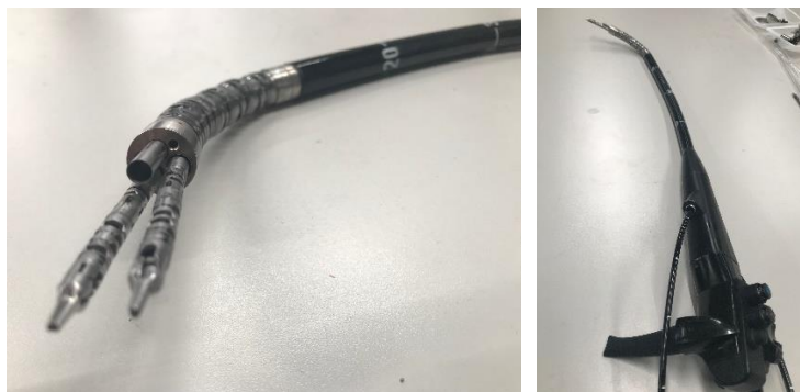
Fig 1.4 Endoluminal surgical system; Two flexible surgical instruments guided internally, by two channels inside an overtube. Another channel is dedicated for imaging device, and a small independent channel for irrigation. An overtube is manually operated to roughly reach the target surgery site.
