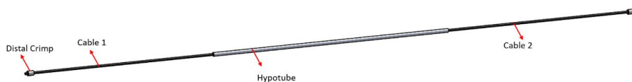
Fig. 1.9 Hypotube reinforced tendon in laparoscopic surgical instruments; tendon will be routed with a pulley to the driving element, at non-reinforced region
