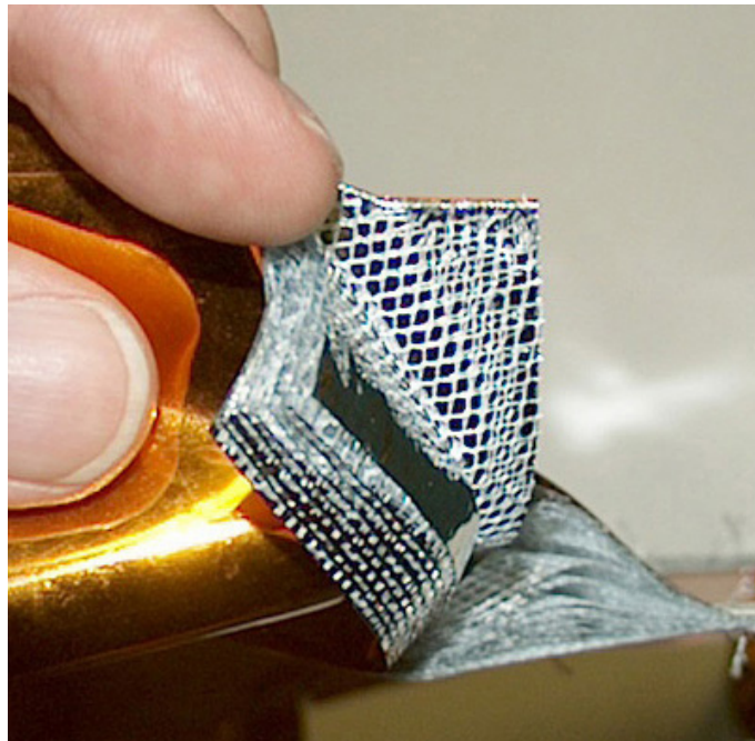
Figure 2.9 Inner Configuration of an MLI [51]
