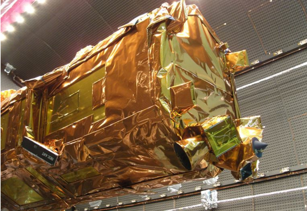
Figure 2.10 MLI installation on a satellite
