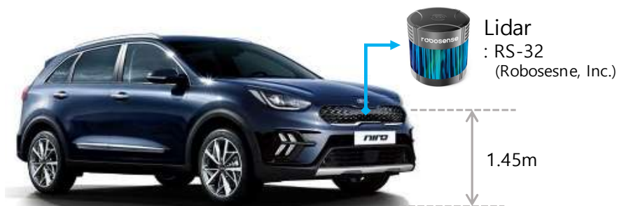
Figure 6.6. Test vehicle and sensor configuration
