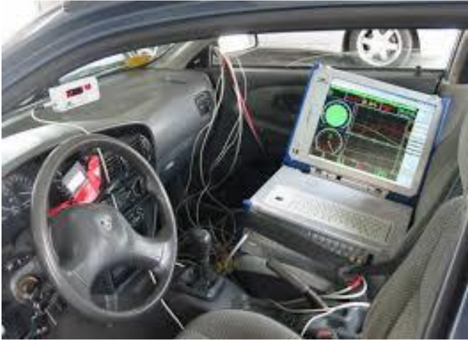
Figure 8.5. The configuration of measurement data acquisition system.
