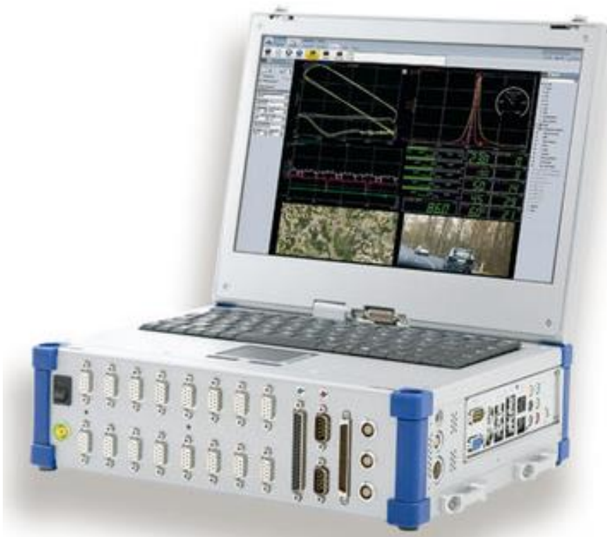
Figure 8.4. Data acquisition system, DEWE-211 (courtesy of DEWETRON GmbH).
