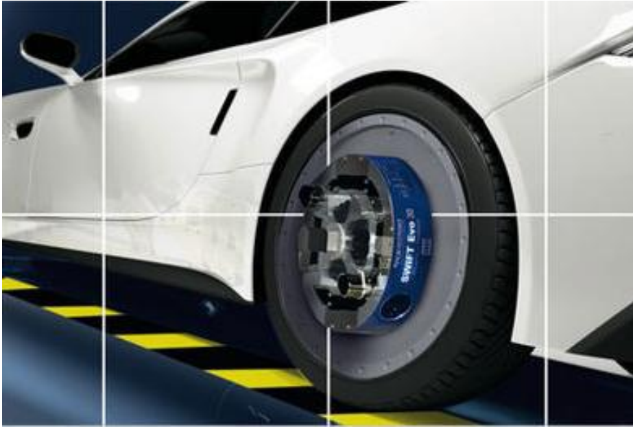
Figure 8.3. The configuration of wheel force transducer system in test vehicle.
