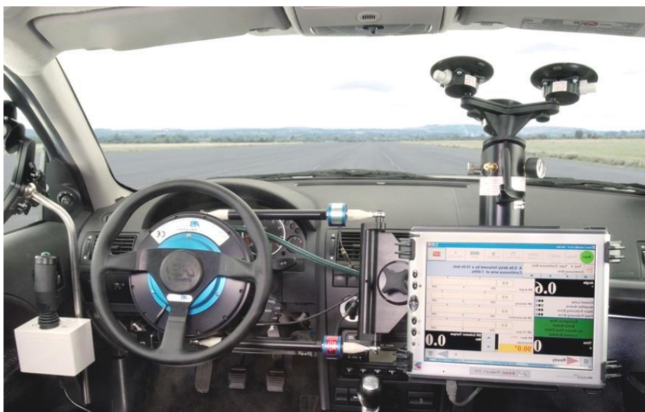
Figure 8.1. The configuration of the test vehicle with steering robot.
