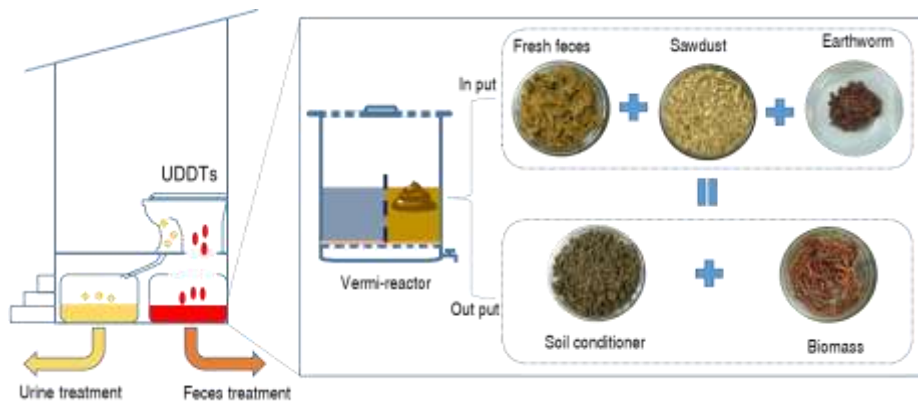
Figure 5. 1 Graphical conclusion of vermicomposting of source-separated human feces with the addition of sawdust
