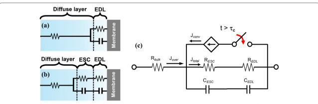
Fig. 4 Schematics of equivalent circuit of ICP layer at a ohmic current regime and b overlimiting current regime. c A unified equivalent electrokinetic circuit model of ICP layer considering EDL, ESC and 2nd EOF
