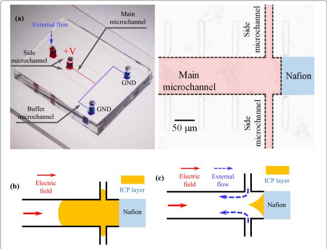
**Fig. 1** a Image of micro/nanofluidic device used in this work and the magnified view of the device. Main and buffer microchannel had the dimension of 15  $\mu$ m depth  $\times$  100  $\mu$ m width and the side microchannel had one of 15  $\mu$ m depth  $\times$  150  $\mu$ m. The ICP layer **b** without or **c** with external flow from two side microchannels
