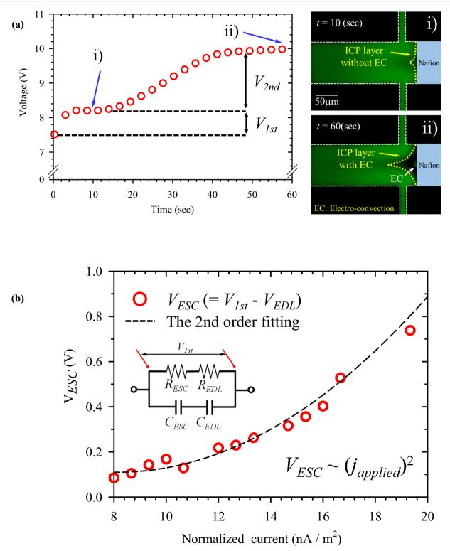
**Fig. 3** a The result of chronopotentiometric measurement at 29 nA (in the regime of OLC regime) and the corresponding images at i) t = 10 s and ii) t = 60 s, respectively. **b** The  $V_{1st}$ - $i_{applied}$  relations and the equivalent circuit model of the ICP layer at inset of the graph
