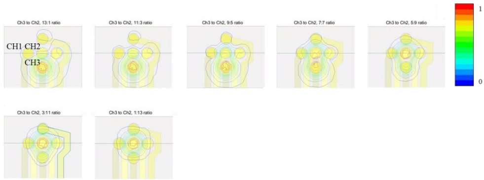
Figure S.2.5 FEA results of the steered electric field measurements using the pentapolar stimulation when the recording distance from the stimulation electrodes was 200 \mu\text{m} .
