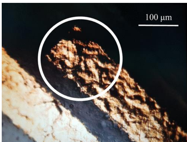
Figure 3.1.2 A microscopic image of a gold channel of the COP-based depth-type microprobe. The geometrical surface area of the channel was 100×100 μm, though its effective surface area would be larger because of the rough surface of the gold thin film.
