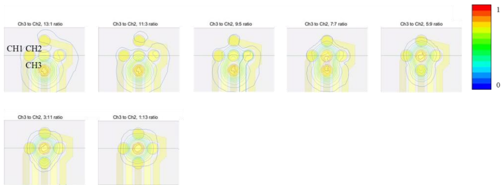
Figure S.2.6 FEA results of the steered electric field measurements using the pentapolar stimulation when the recording distance from the stimulation electrodes was 250 \mu\text{m} .
