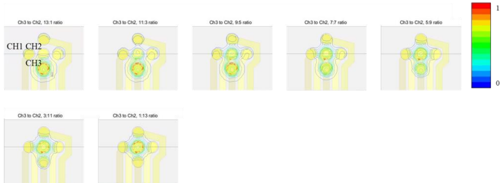
Figure S.2.1 FEA results of the steered electric field measurements using the penta-polar stimulation when the recording distance from the stimulation electrodes was 13\ \mu\text{m} .
