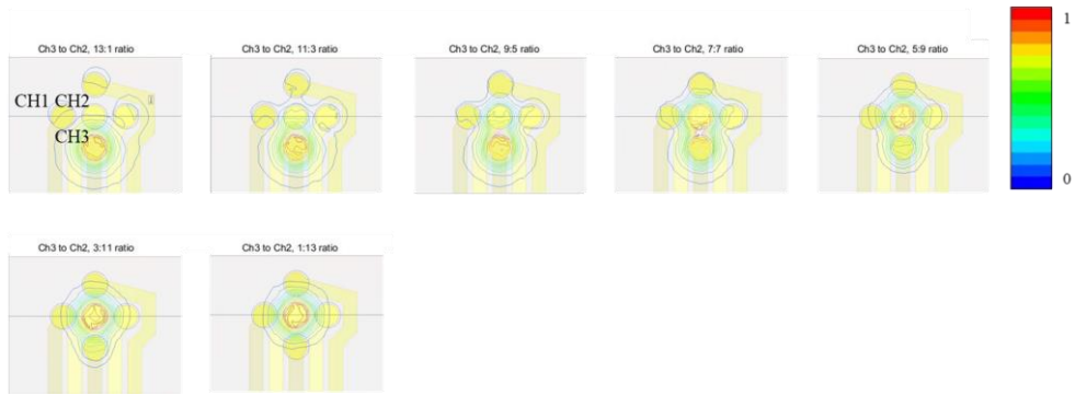
Figure S.2.3 FEA results of the steered electric field measurements using the pentapolar stimulation when the recording distance from the stimulation electrodes was 100 \mu\text{m} .
