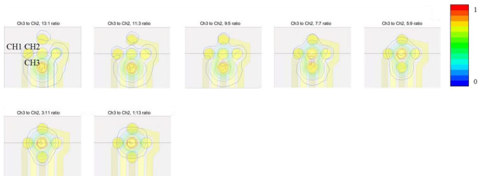
Figure S.2.4 FEA results of the steered electric field measurements using the pentapolar stimulation when the recording distance from the stimulation electrodes was 150 \mu\text{m} .
