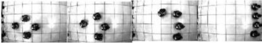
(a) Robot formation switch from diamond to line, Images from [68]
