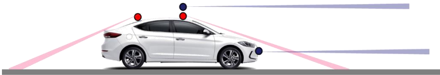
(a) Side view of four lidar sensors installation
