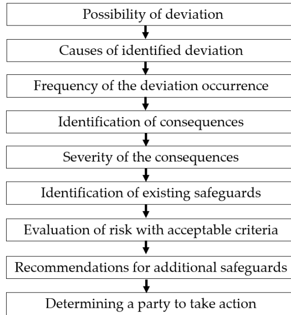
Figure 7. The steps used in hazard identification from derived deviations (adapted from Macdonald, 2004).
