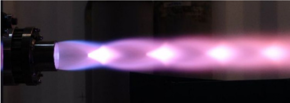
Figure 1.19. Shock diamonds in a flow exiting a nozzle in an aircraft taken from https://www.zmescience.com/other/science-abc/diamond-rings-aircraft-0423423/ .
