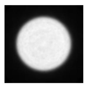
Figure 5-11. Reconstructed uniform phantom image.
