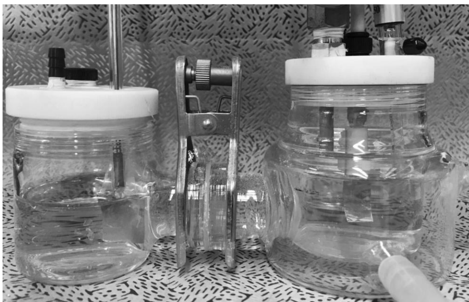
Figure 2.3. Image of the H-type cell for electrochemical reduction of N_2O .
