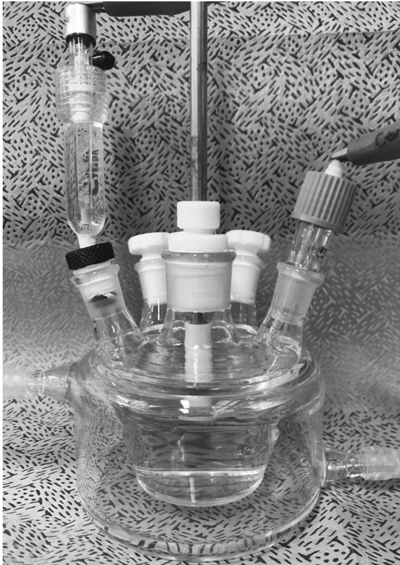
Figure 2.1. Image of the three-electrode system for electrochemical analysis of the prepared catalysts.
