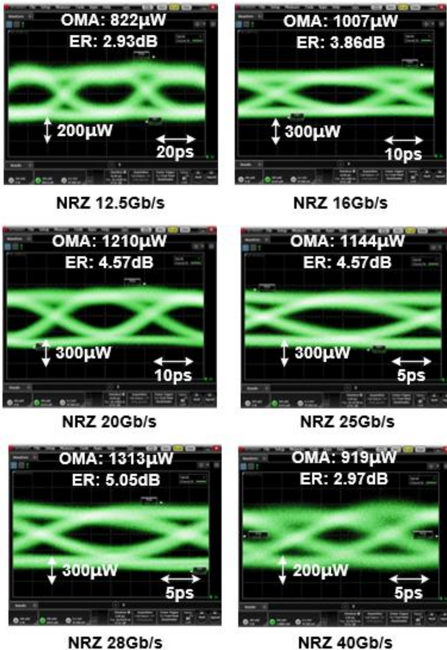
Fig. 4.8. Optical eye diagrams of NRZ data from 12.5Gb/s to 40Gb/s.
