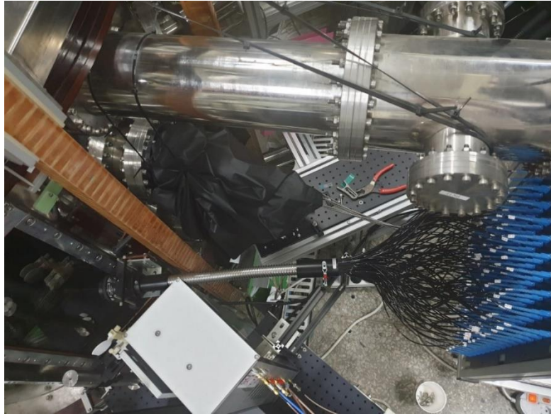
Figure 2-6 Collecting optics including collecting lens, fiber bundle, and patch panel.
