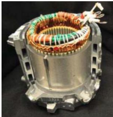
Fig. 1.4 Water cooling jacket of Nissan Leaf motor [6]
