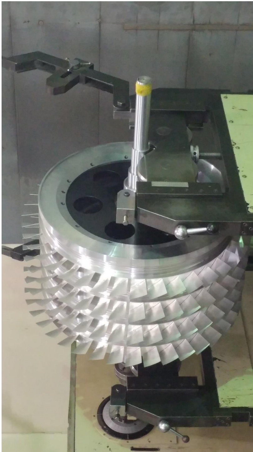
Figure 2.21 Picture of Compressor Rotating Parts Installed at a Balancing Machine
