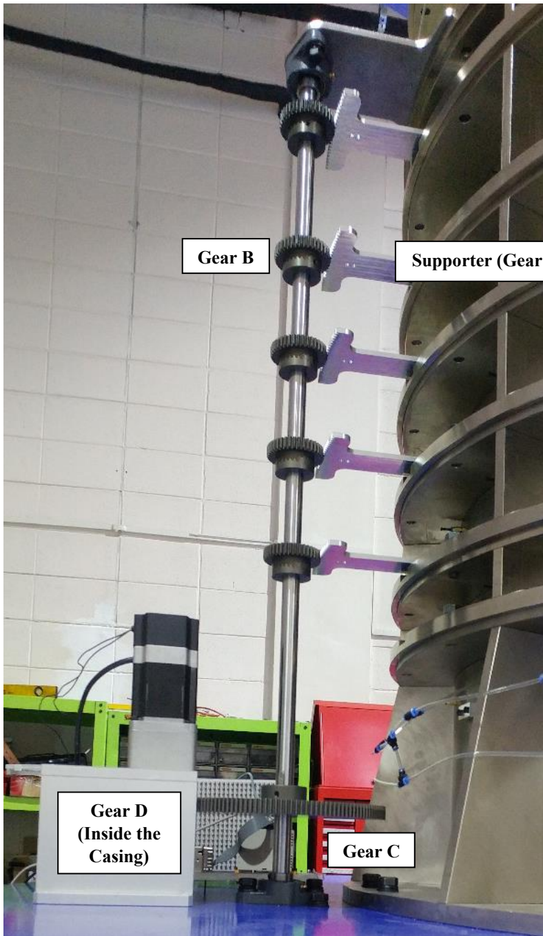
Figure 2.26 Circumferential Traversing System of SNU Compressor
