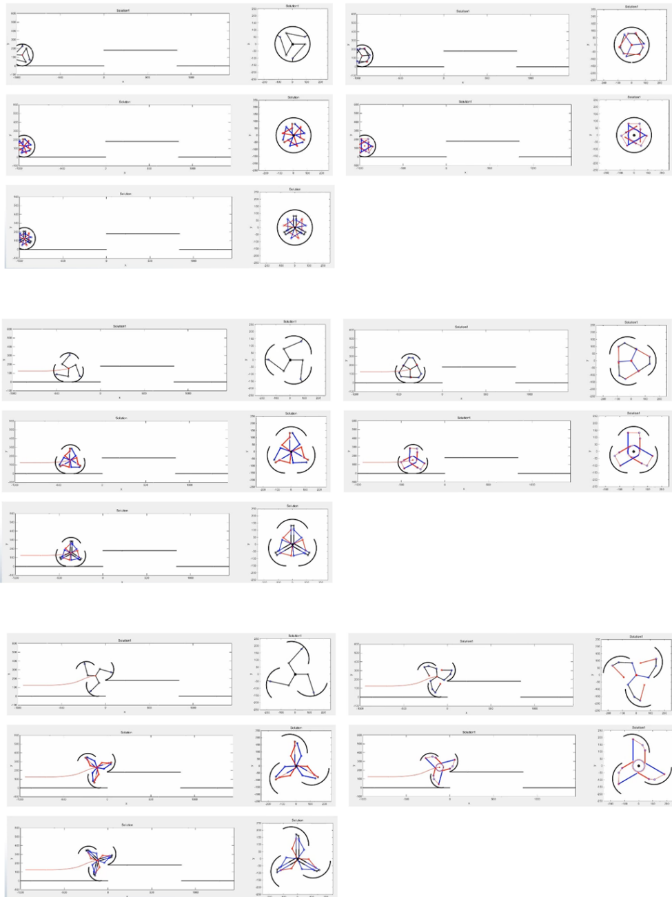
Figure 3.22. Step overcoming simulation results (1/2) for 5 design alternative mechanisms
