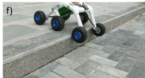
Figure 1.5. Step climbing process of the rocker bogie mechanism
