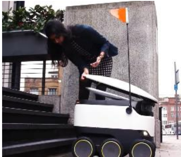
Figure 1.2. Limitations of Existing Service Robot Driving Platform - A person must come down the stairs and get goods
