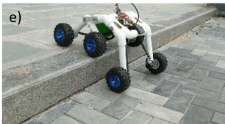
Figure 1.5. Step climbing process of the rocker bogie mechanism
