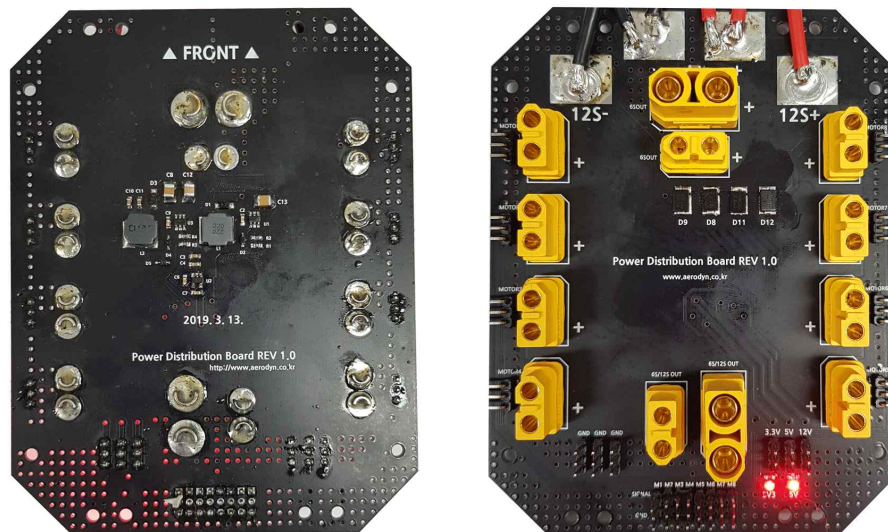
Fig 25. Power Distribution Board for BLDC Motor System
