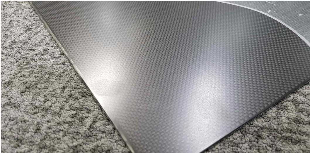
Fig 13. Plate of 3K Plane CFRP (Thickness : 2mm)
