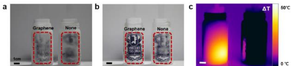
Figure 4. Optical and IR photographs showing the EM-induced defogging of graphene coated vials. (a) The photograph before applying EM waves. Left is the graphene-coated bottle and right is the none-coated bottle. (b) The photograph after applying microwave during 5 s. (c) An infrared picture immediately obtained after microwave irradiation. Scale bars, 1 cm.
