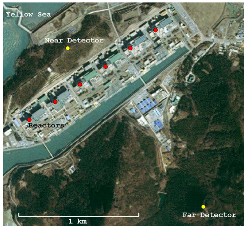
Figure 2.3: Layout of the Hanbit experimental site. The red dots and yellow dots represent reactors and detectors, respectively. Six reactors are spaced approximately equally in a 1280 m span. The near and far detectors are located at a distance of 290 m and 1380 m from the reactor array, respectively. The image taken from Google Earth™ and copyrighted therein. © 2015 Google, DigitalGlobe
