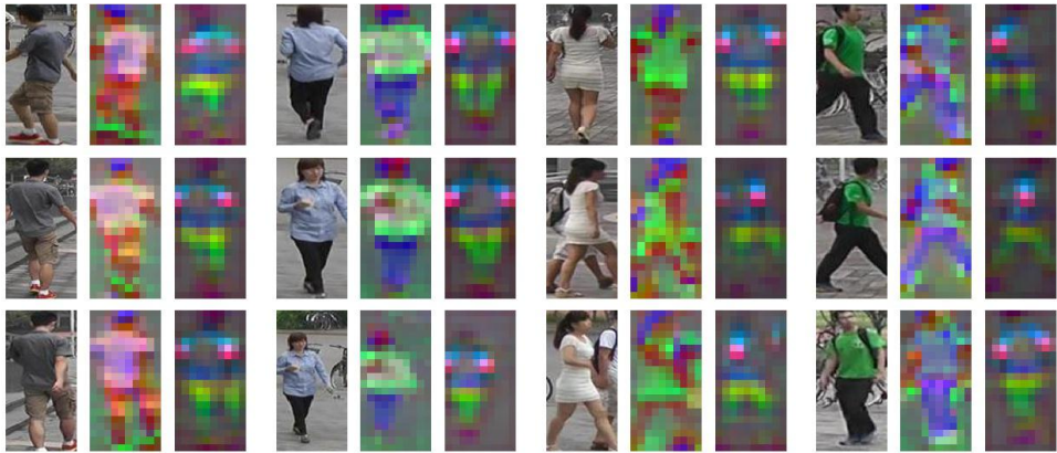
Figure 2.3: Visualization of the appearance maps \mathbf{A} and part maps \mathbf{P} obtained from the proposed method. For a given input image (left), appearance (center) and part (right) maps encode the appearance and body parts, respectively. For both appearance and part maps, the same color implies that the descriptors are similar, whereas different colors indicate that the descriptors are different. The appearance maps share similar color patterns among the images from the same person, which means that the patterns of appearance descriptors are similar as well. In the part maps, the color differs depending on the location of the body parts where the descriptors came from. (Best viewed in color)
