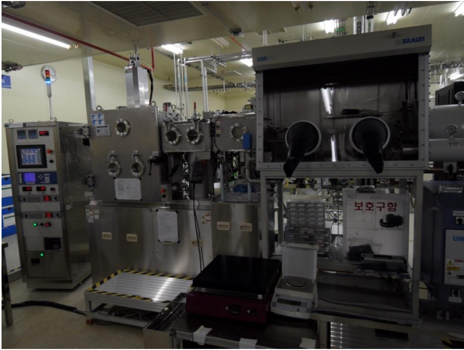
Figure 1.11 A thermal evaporator located at the Inter-University Semiconductor Research Center of Seoul National University.
