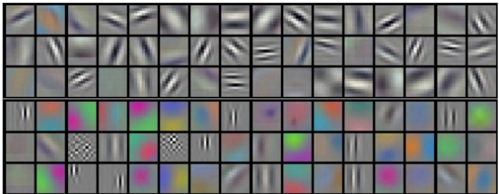
Figure 6: Spatial features from input images learned by CNN filters.
