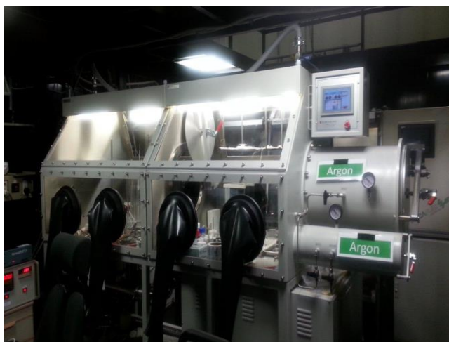
Figure 5.1 Glove box for electrochemical experiments
