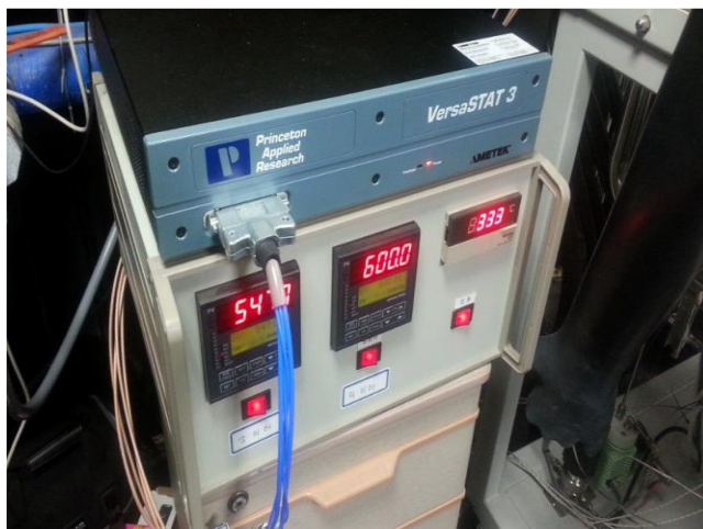
Figure 5.2 VersaSTAT3 potentiostat and PID heater controller
