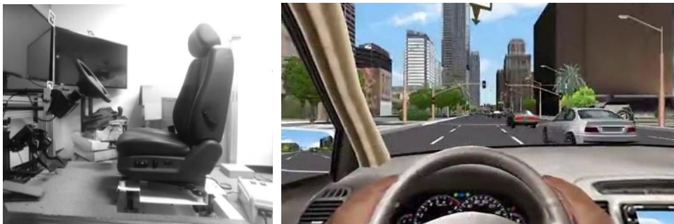
Figure 1. An adjustable vehicle mock-up and driving simulation software
