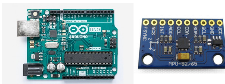
FIGURE 4.2: MPU-9255 (IMU sensor for getting the information of acceleration and yaw angular velocity) and Arduino Uno for sending the information from the IMU to computer (NUC7i7) and the velocity input to the motor set
