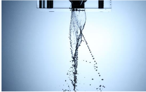
Figure 4.4 Spray images of the liquid injector when the lip thickness of the gas injector is 3.8 mm
