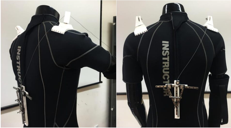
Figure 5. (Left) The side view of the overall wearable component of the device. (Right) Rear view of wearable component and actuator. A bearing is embedded so that horizontal movement of upper body will not cause derailment of the force transmitting tendon.
