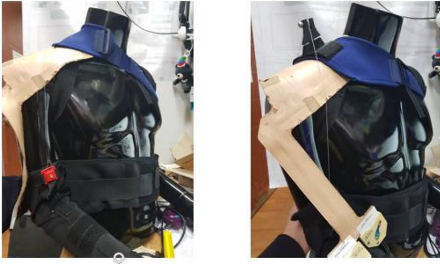
Figure 11. (Left) The experiment setup with no MA structure. The compression is measured with Novel pressure pad placed on top of the shoulder of the mannequin. (Right) The experiment setup with the proposed MA structure. Same setup is applied except for the addition of moment arm structure on top of the shoulder.
