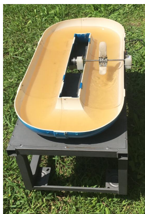
Fig. 11. Low-cost, homemade raceway pond reactor. Source: Author.
