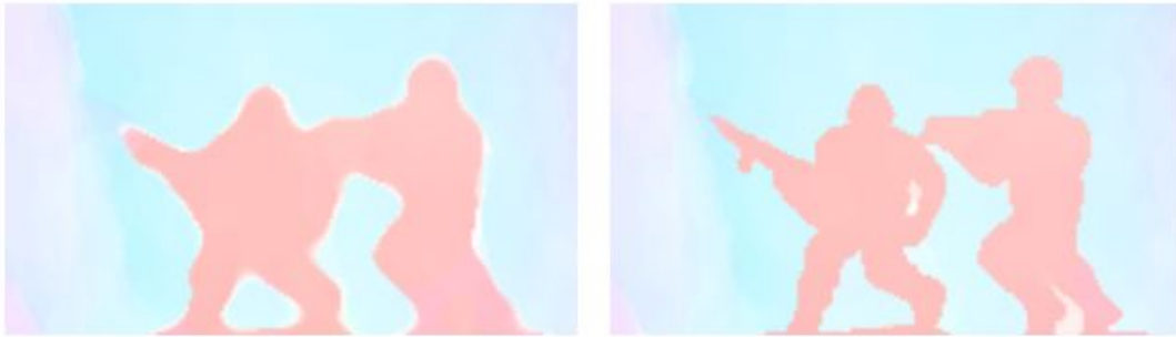
Figure 2.4: Median filtering over-smoothes the rifle in the “Army” sequence, while the proposed weighted non-local term preserves the detail. Results of (a) Classic++ (b) Classic+NL (Source: Sun, Roth and Black (2010))
