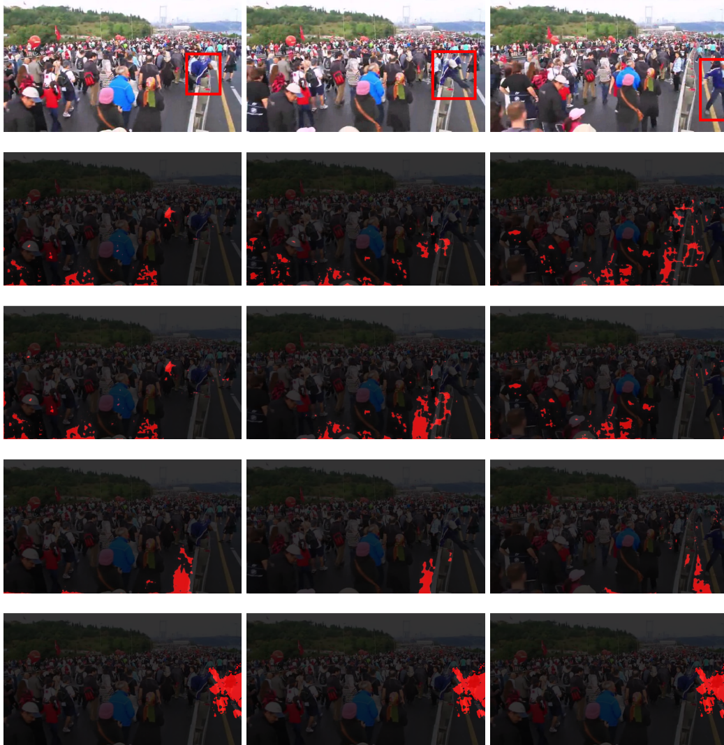
Figure 4.17: Anomalies detected in 1_34_008681798-people-walk-europe-3 scene of CUHK dataset using RNN. First row shown the reference frames - 50, 60 and 81 -, the second row shown results with T = 1 , the third row T = 1 plus our post-processing method, the fourth row T = 14 and the last row T = 100 .
