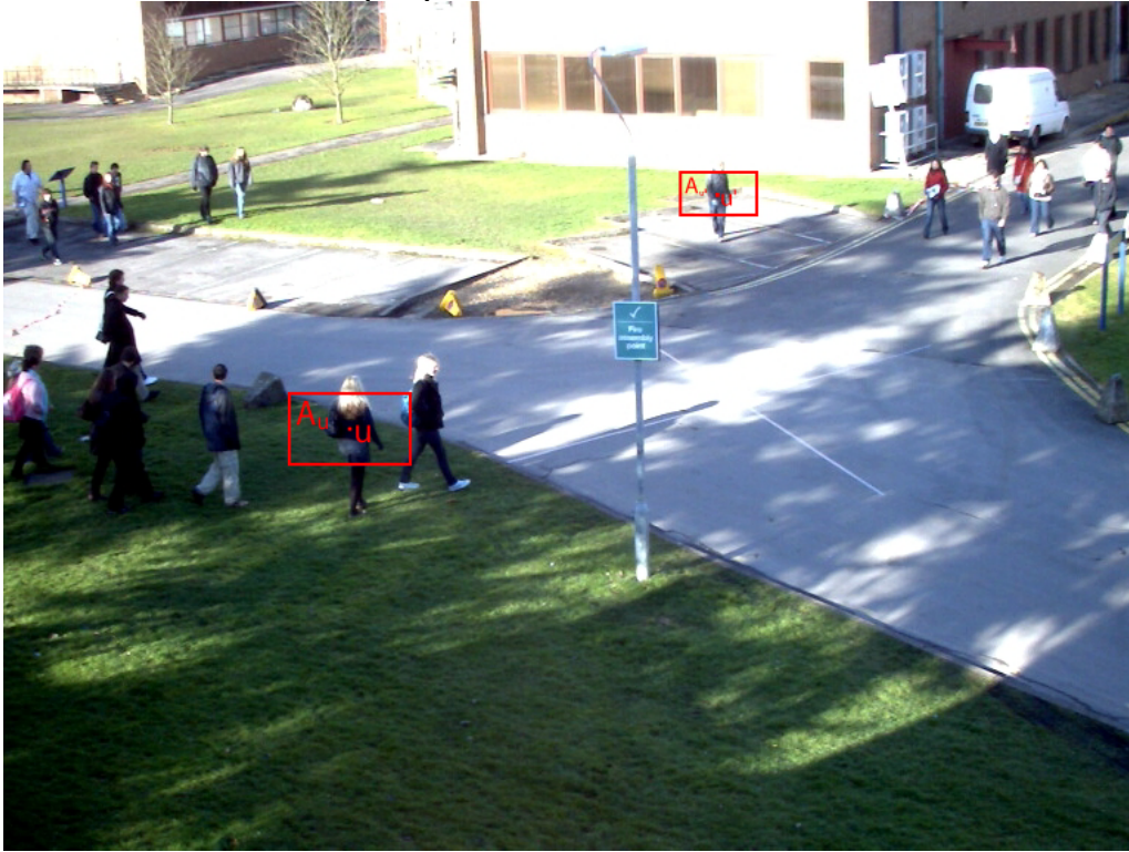
Figure 3.2: Example of a “region of influence” with the same size in world coordinates projected back to the image at different pixel locations. In the image domain they present different sizes, due to camera perspective.
