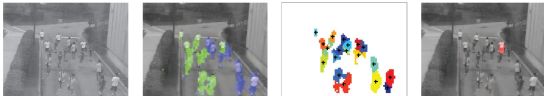
Figure 2.10: Pipeline of the method proposed by Jiang et. al (a) Original video frame (b) Patch classification (c) Blob representation (d) Contextual anomaly (Source: (JIANG; WU; KATSAGGELOS, 2009))
