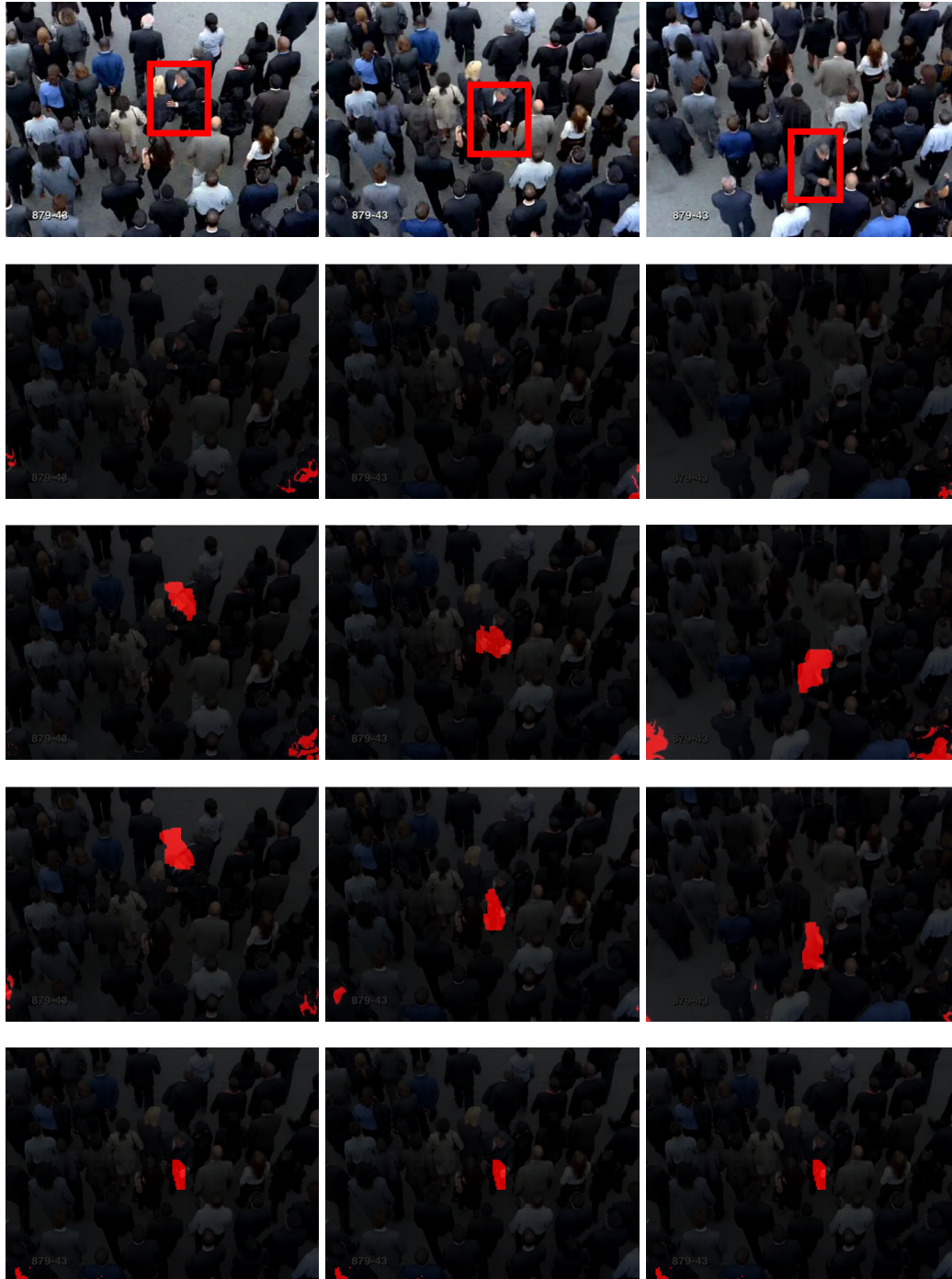
Figure 4.22: Anomalies detected in scene 1_879-43_1-2 of CUHK dataset using SVM model. First row shown the reference frames - 50, 62 and 98 -, the second row shown results with T = 1 , the third row T = 1 plus our post-processing method, the fourth row T = 14 and the last row T = 100 .
