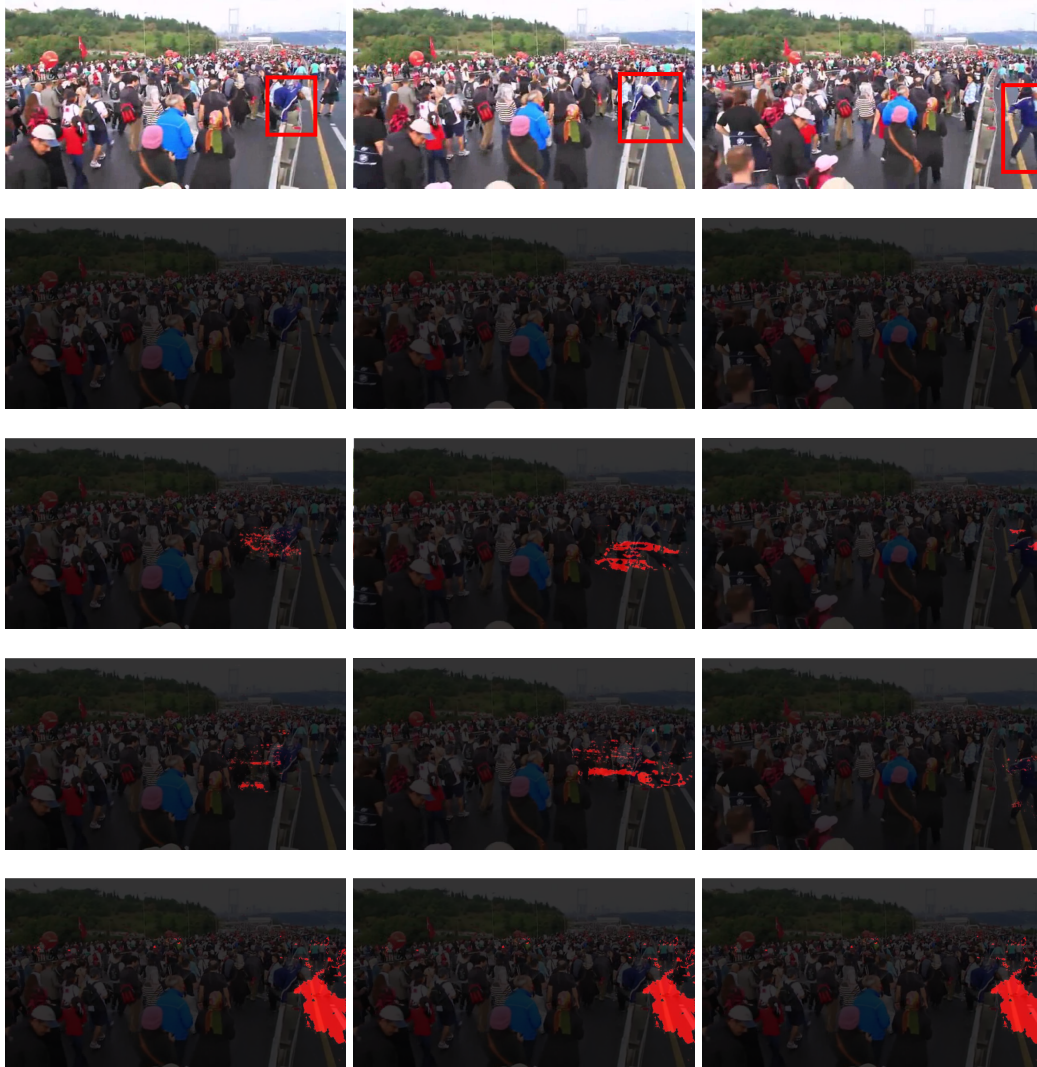
Figure 4.18: Anomaly detection results of scene 1_34_008681798-people-walk-europe-3 CUHK dataset using SVM model. First row shown the reference frames - 50, 60 and 81 -, the second row shown results with T = 1 , the third row T = 1 plus our post-processing method, the fourth row T = 14 and the last row T = 100 .
