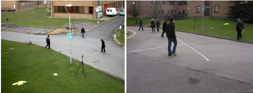
Figure 1.4: Same scenario filmed by two cameras. The distance in image coordinates between people are different in each scene. (Source: PETS2009 (FERRYMAN; SHAHROKNI, 2009))
