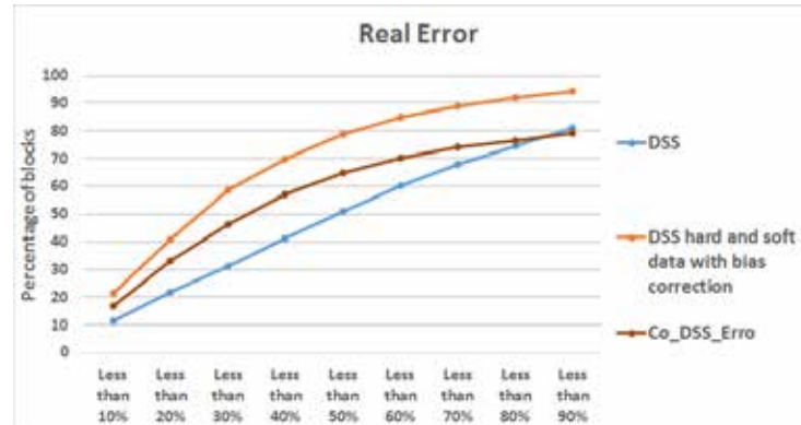
Figure 6- Real error in block using the reference block model for comparison between the methodologies a) Direct Sequential Simulation with only hard data b) Direct Sequential Simulation with hard and soft data with bias correction c) Direct Sequential Cosimulation with hard and soft data
