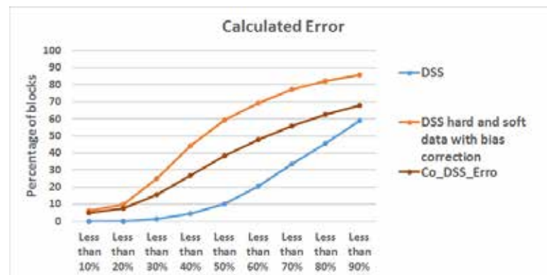
Figure 7- Calculated error of block using the reference block model for comparison between the methodologies a) Direct Sequential Simulation with only hard data b) Direct Sequential Simulation with hard and soft data with bias correction c) Direct Sequential Cosimulation with hard and soft data
