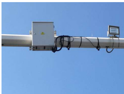
Fig 5. RSU components used in the V2X trials in China twinning project. The message exchange benefits between RSU and in-vehicle OBUs are the trial goals.
