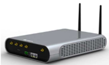
Fig 5. RSU components used in the V2X trials in China twinning project. The message exchange benefits between RSU and in-vehicle OBUs are the trial goals.
