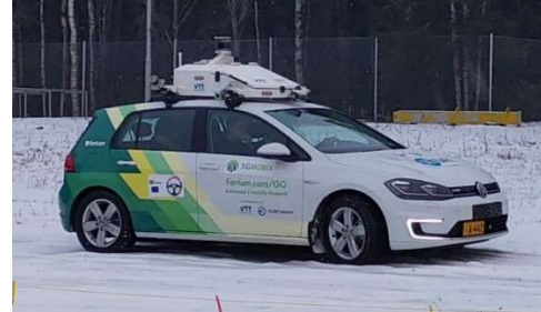
Fig 1. eLvira remotely operated and automated passenger car used in the European V2X trials.
