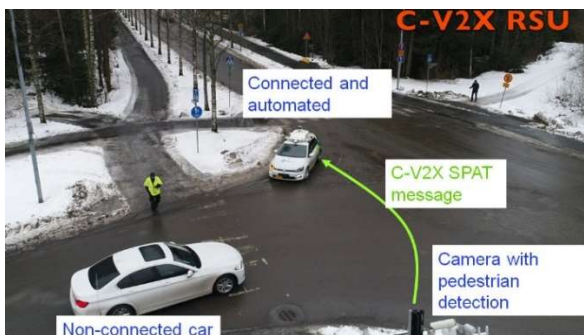
Fig 4. eLvira remotely operated and automated passenger car for V2X trials. One of the key targets is to enable low latency intersection driving support functionality where RSU and connected vehicles can cover all blind spots.
