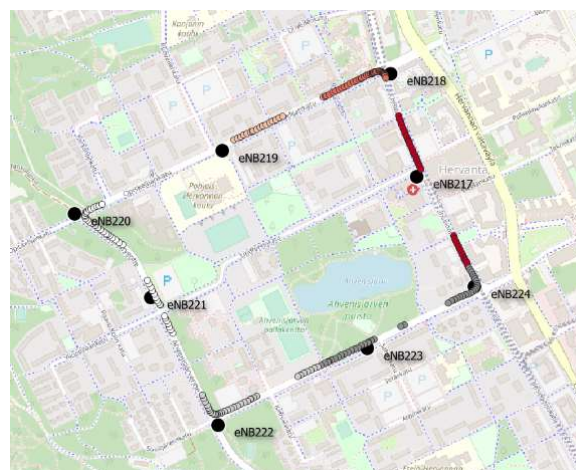
Fig 8. eNB locations and RSRP > -90dBm in European test site. There are 9 base-stations in the area.
