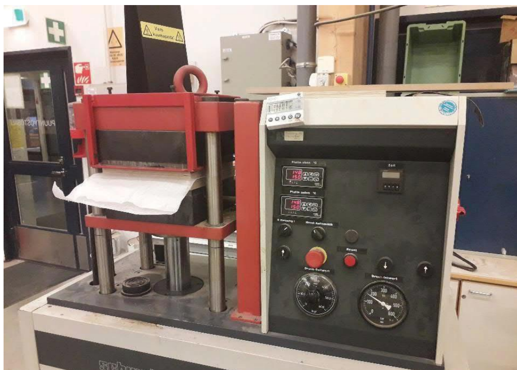
Figure 52 Polystat s 200. The plate size 250 mm x 250 mm (Xamk Wood Laboratory)
