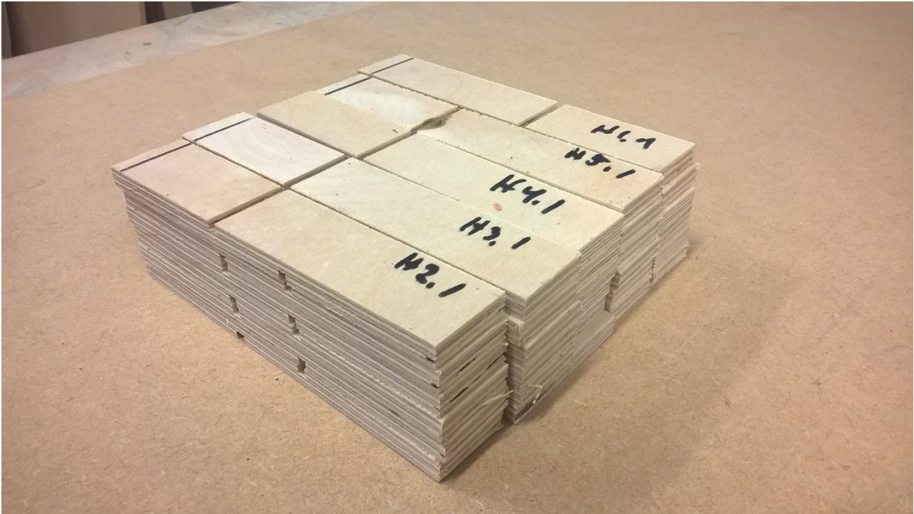
Figure 49 EN 314-1 test pieces
