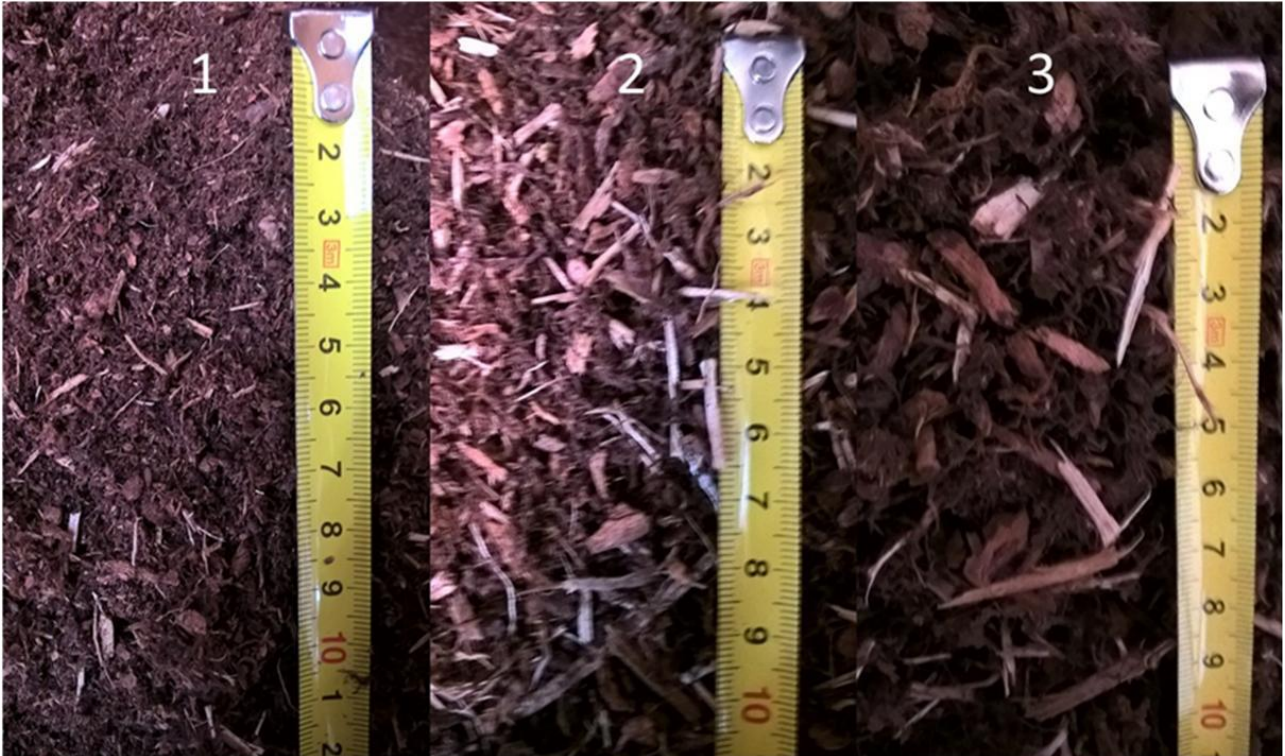
Figure 10 Three fractions obtained by use of vibrating slope screen
