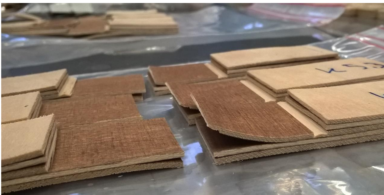
Figure 51 Experimental tannin-resin after water immersion and shear test
