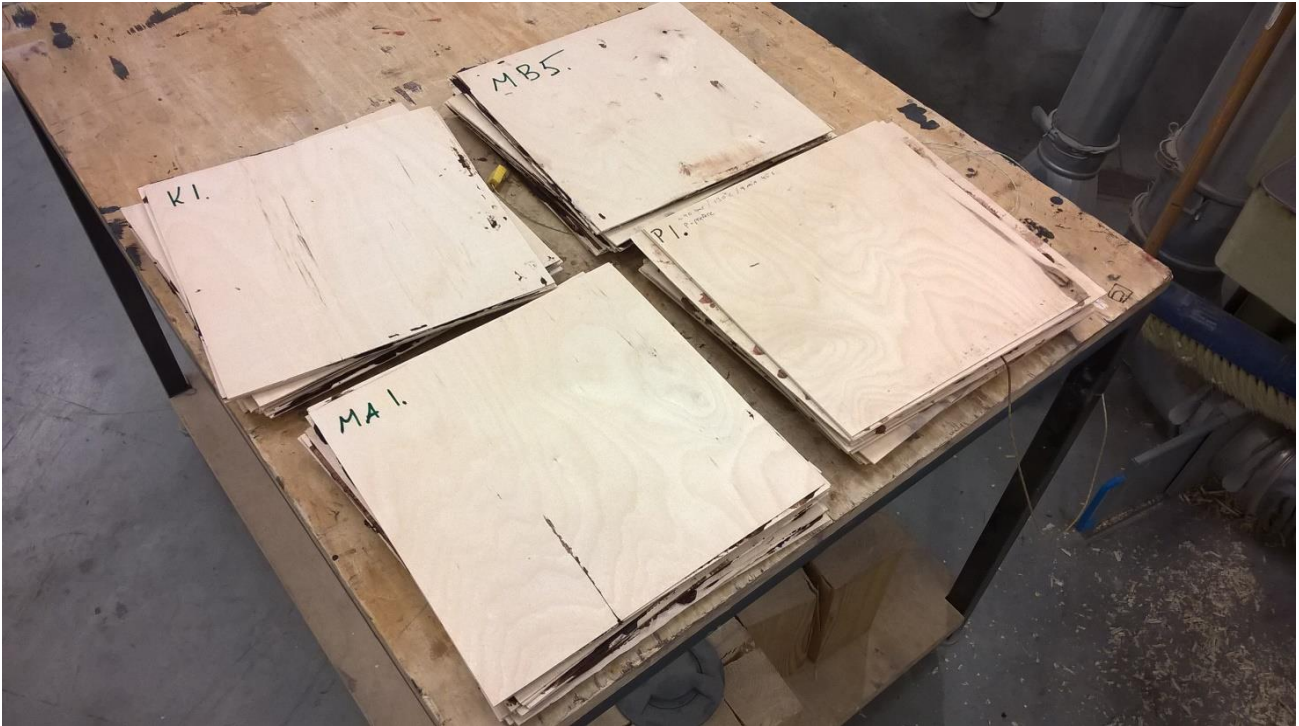
Figure 48 Test panels (5 ply; 250 mm x 250 mm)
