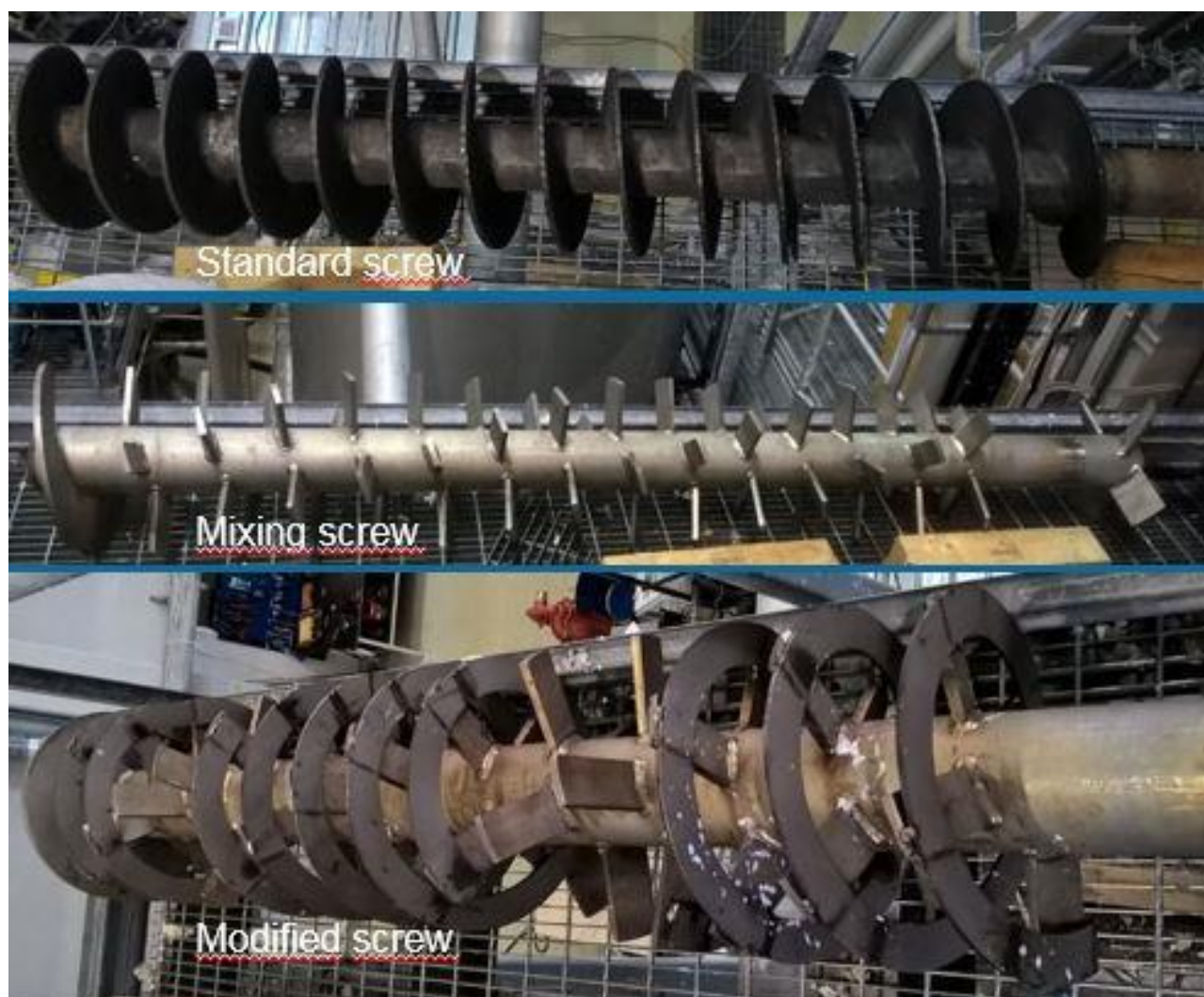
Figure 12 The screw types used in continuous screw reactor during the experimental runs
