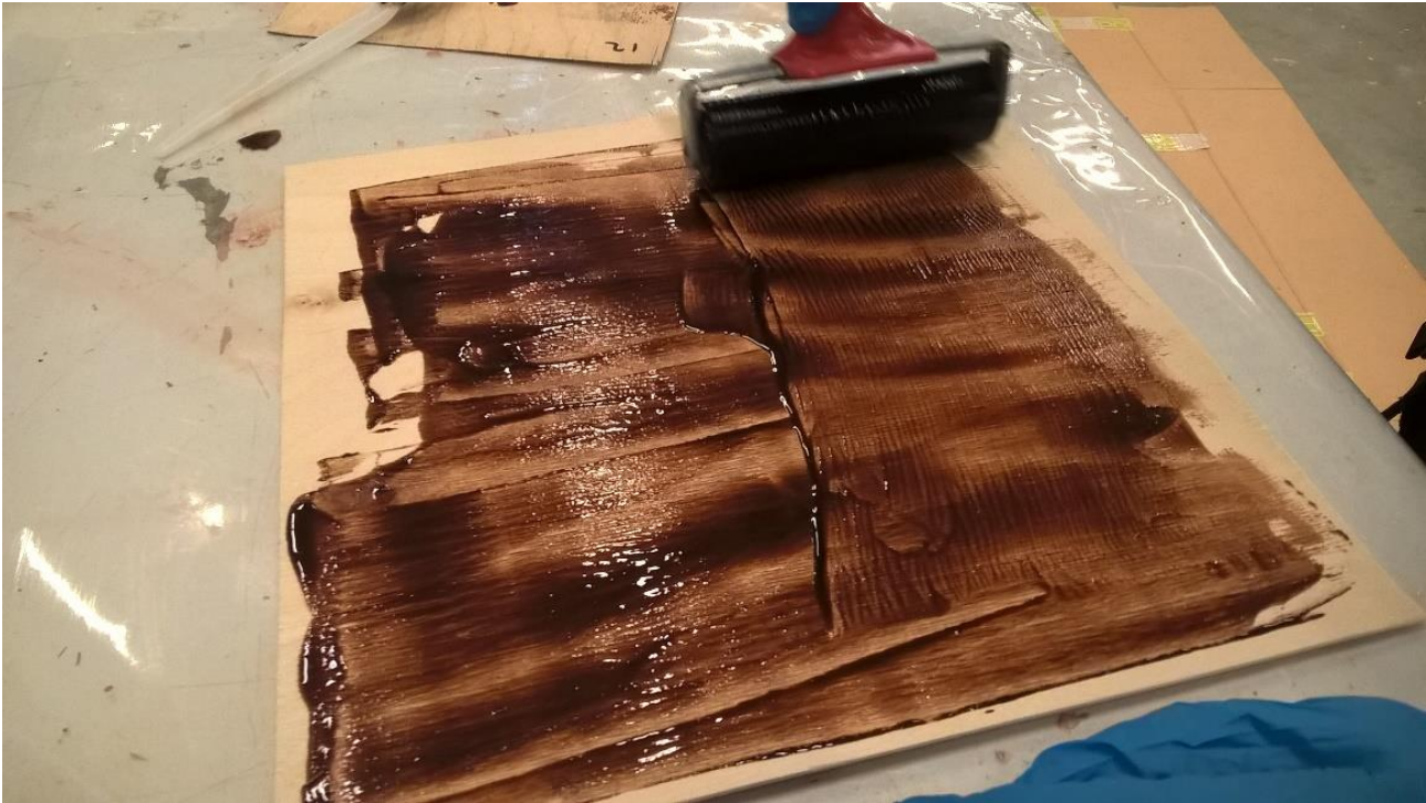
Figure 47 Glue application by hand (rubber roller)
