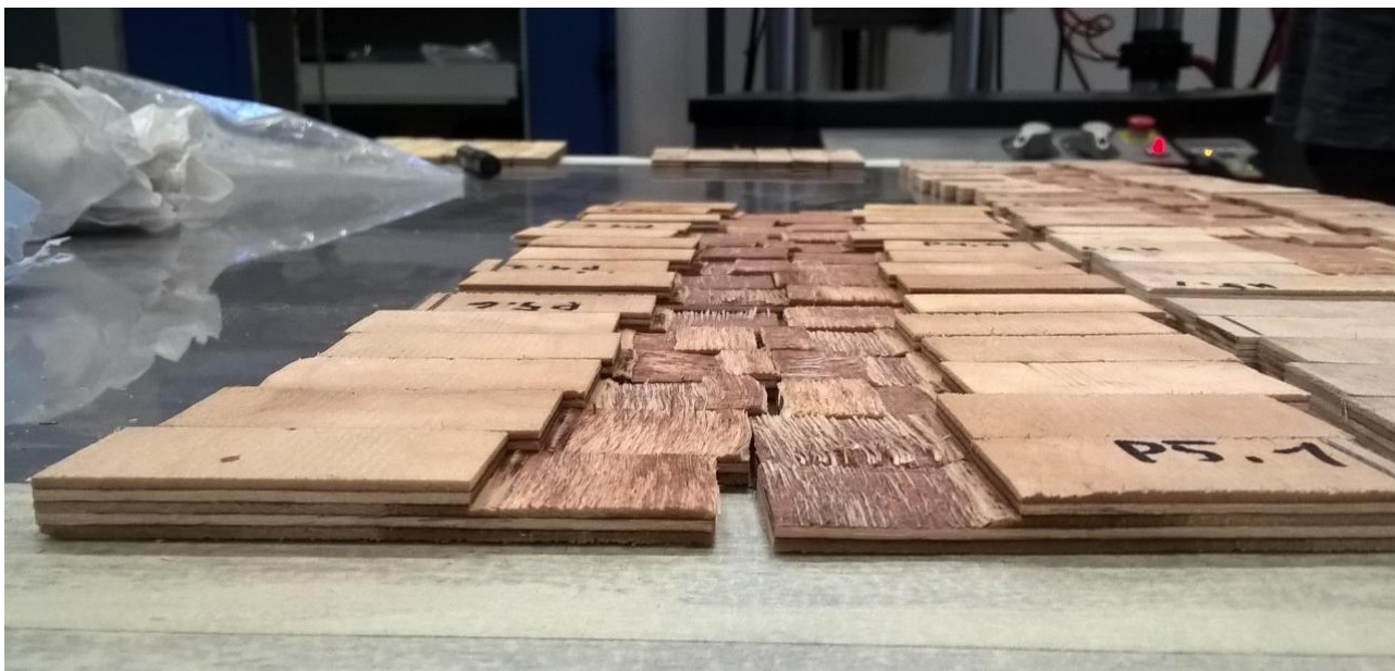
Figure 50 Commercial resin after water immersion and shear test
