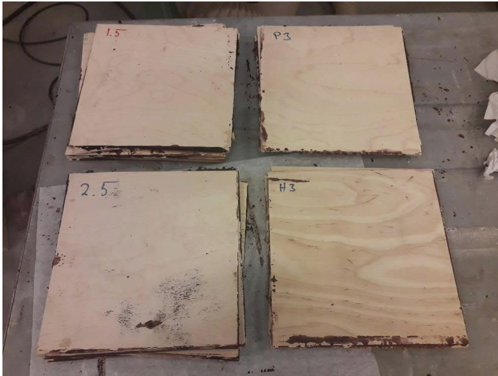
Figure 54 Test panels (5 ply; 250 mm x250 mm)
