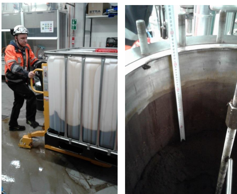
Figure 20 Hot water extract in a container and extracted bark remaining in the vessel
