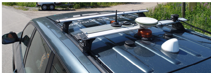
Fig. 2. 4G and GNSS antenna setup on roof of the test vehicle Martti with V2X capable antennas.
