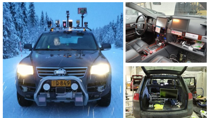
Fig. 1: The instrumented test and development vehicle Martti with the sensors installed on the roof.
