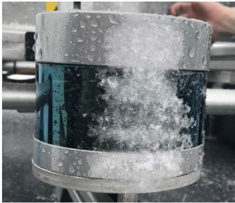
Fig. 13: Frozen LiDAR sensor causes disturbance to the measurements and blocks the laser beam.
