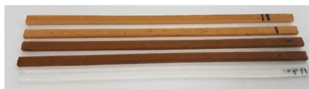
**FIGURE 1** Appearance of aging test specimens (from bottom) REF, UH-REF, UH-EL, BH-REF, BH-EL [Color figure can be viewed at wileyonlinelibrary.com]
