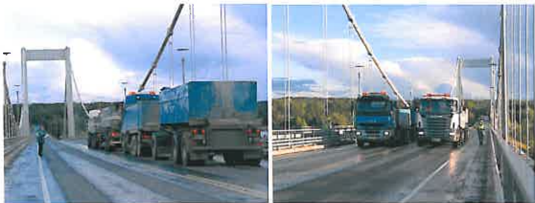
Figure 10.1.1. The heavy lorries used in the loading test in Kirjalansalmi bridge in 2007.
