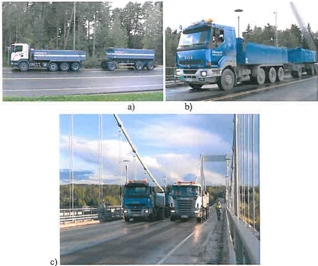
Figure 3.3.5. Vehicles used in the loading test in 30.8.2008. a) Vehicle No 1, b) vehicle No 2 and c) vehicles in the loading test 1F.
