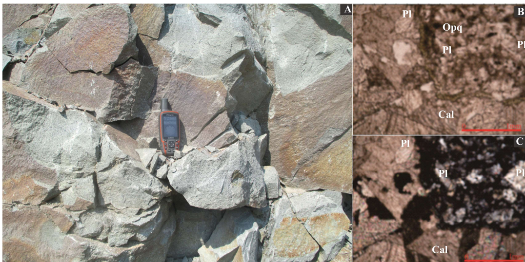
FIGURE 6. Photographs of slightly weathered andesite: (A) Outcrop; (B) Thin sections of SW1 sample under PPL and (C) XPL.
