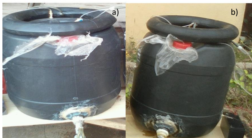
Figure 1 a) Conventional digester and b) electrolyzed digesters
