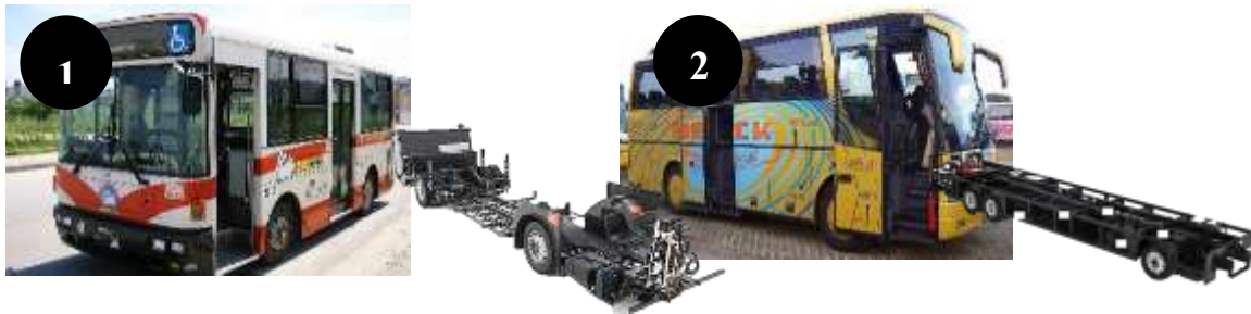
Gambar 2. 3. (1) low floor bus dan chassis (2) High Floor bus dan Chassis
