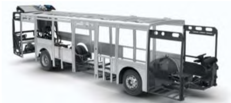
Gambar 2. 29. Rangka Bus Vovlo Electric Hybrid
