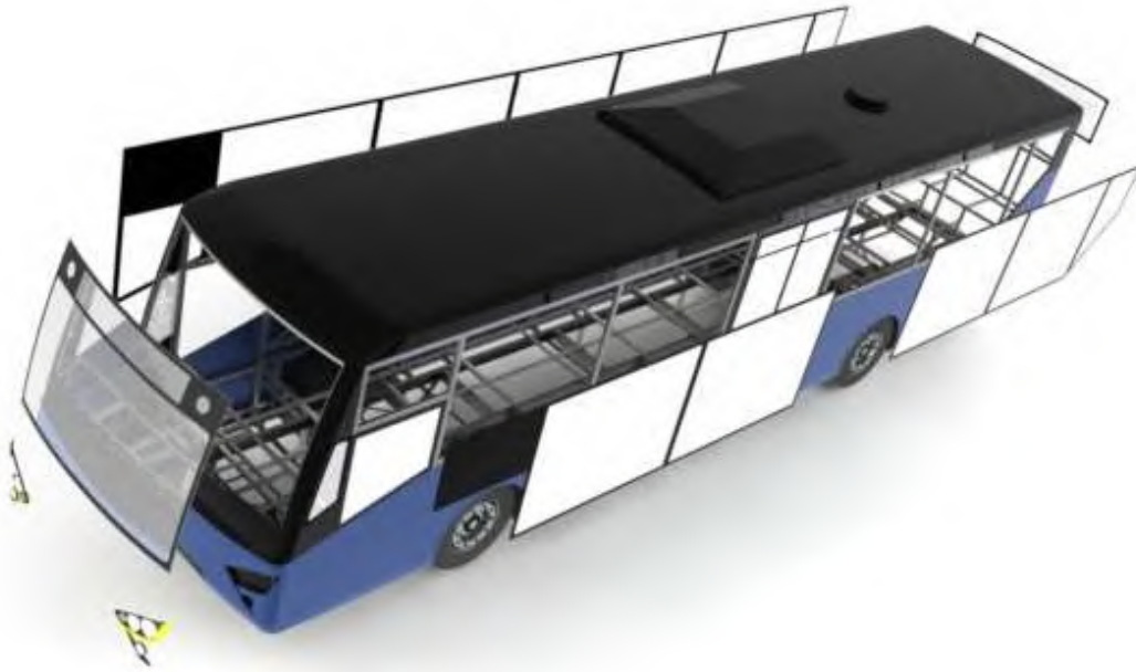
Gambar 5. 31. Proses Assembly Kaca
