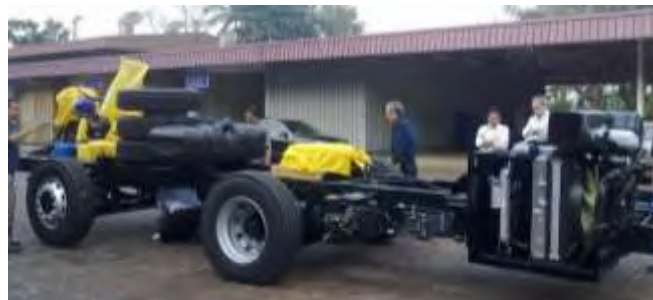
Gambar 2. 6. Chasis Modular bus Scania
