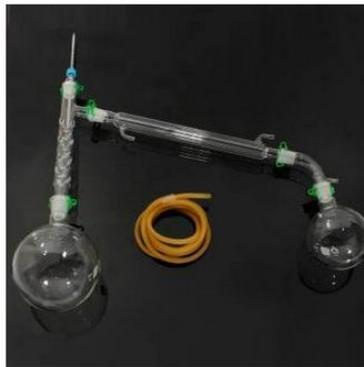
**Gambar 3.4** Unit Hidrodestilasi
